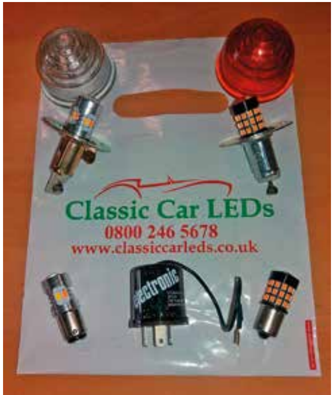
Frogeye setup – note the combined amber/white bulbs BAY15D for the front. Later cars just need 4 amber BA15S bulbs.
