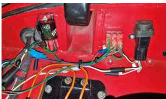
To the right of the new hazard switch is an inertia switch for the electric fuel pump.
