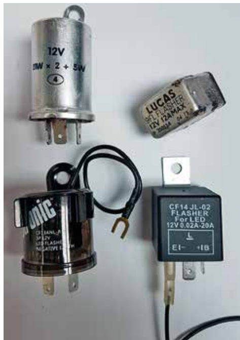
Modern flashers below the bimetallic types. Note the extra earth wire on the modern flashers and large pipe clip used to secure the round type.
