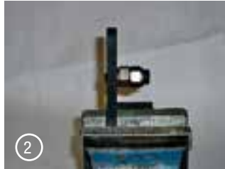
Photo 1 Showing bolt set to required length and secured ready for sawing.
