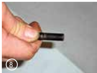
Photo 7 Hand chamfering first thread of bolt.
