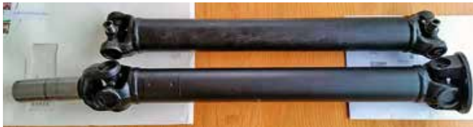
BRB’s old and new (balanced) propshaft: yes, that is the dining room table; a closer look reveals the balance-weight on the left of the shaft.
