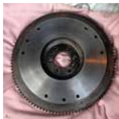
Flywheel skimmed, lightened & balanced
