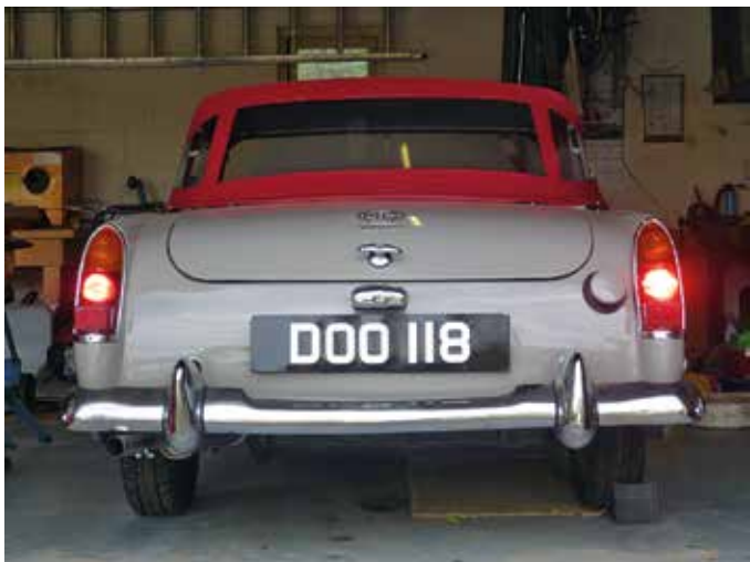
The BAY15D RED STOP/TAIL LED from Classic Car LEDs ( www.classiccarleds.co.uk ) consumes 1/3 the power and gives a noticeably brighter light than the standard filament bulb (Left). This excellent product is a direct replacement for the original.
