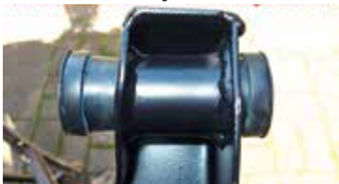
New w/bone with incorrect shape inner bush. Too narrow left hand end. Wider at the right hand end.
