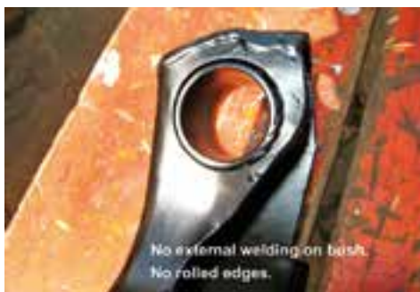
New w/bone with incorrect shape inner bush. Too narrow left hand end. Wider at the right hand end.
