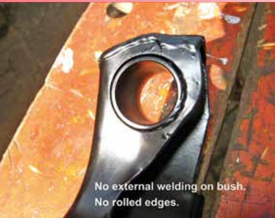
New Moss w/bone with incorrect shape inner bush. Too narrow left hand end. Wider at the right hand end.
