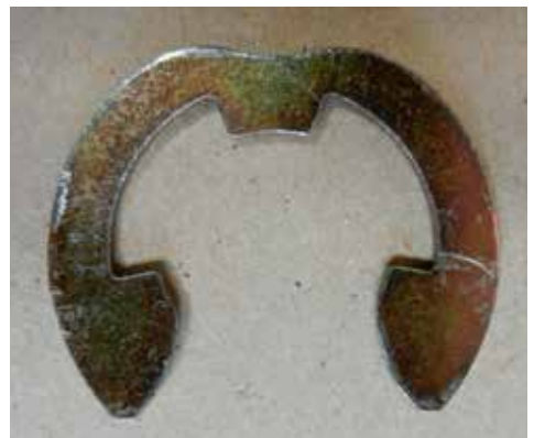
Clip with leading edges filed too"
