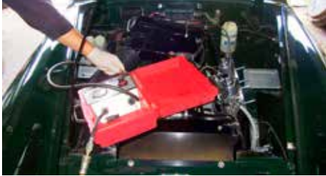
John Wheatley's Midget receives a leak down test
