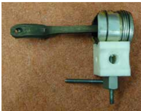
Tool assembled on 1098 piston for pin removal
