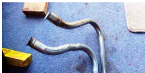
Boa-constrictor pipe (top) with a better one. Mis-shapen exhaust with a better one!
