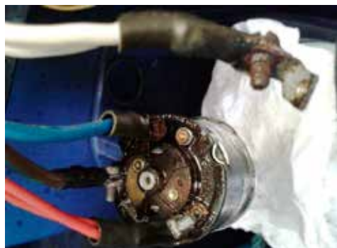
The switch with detached connection
