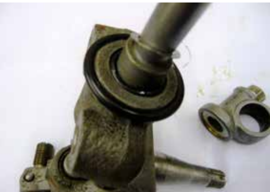
Showing position of optional seal between king pin and upper bush
