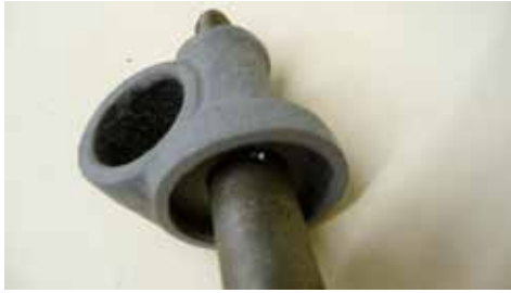
Showing grease outlet hole below trunnion
