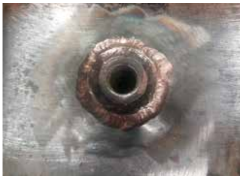
Repaired fuel tank
