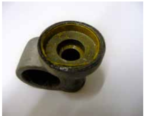
Showing brass shim strip and grease distribution to bearing
