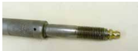
Modified top end with grease nipple and feed hole to bearing
