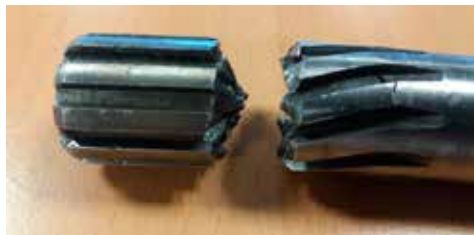
Broken half shaft
