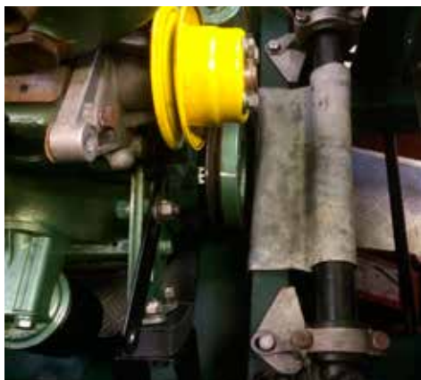
Lead sheet protecting paintwork during engine removal + installation – note timing marks repositioned for sighting from above
