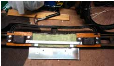
Front bumper with blocks, brackets, foam and number plate fittings, ready to go back in Bridget
