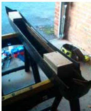
Rear bumper with armature removed and blocks trail fitted. Note the additional plywood needed to gain clearance
