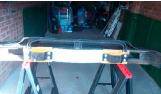
New blocks fitted, void foamed and original brackets screwed home"
