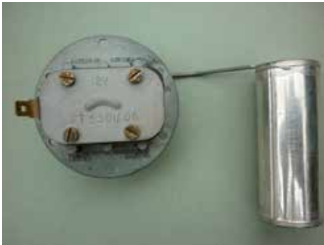
Original tank sender units have serial number FT 5301/06 and a tinned metal float sealed with solder that can rust badly. These senders must only be used with gauges prefixed ‘FG’
