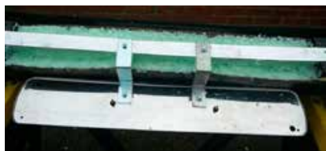
Rear bumper now foamed and covered with GRP. Note aluminium strip screwed to blocks with number plate and brackets
