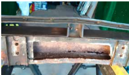
Removing the old armature from the front. Note central section removed to reach upper rivets
