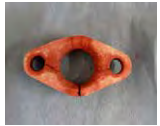
Underside with stain to show cracking
