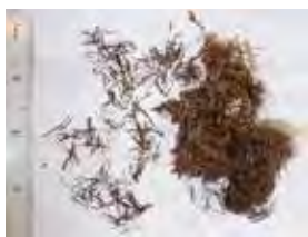
Contents of oil separator
