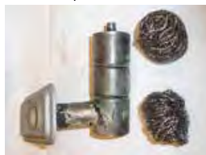
Breather can and proposed packing
