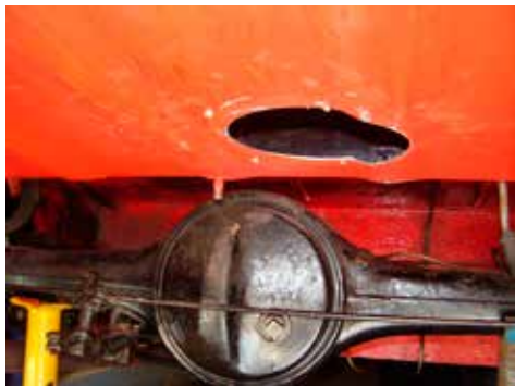
Hole cut into floor
