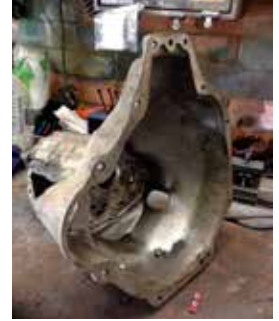
Cut off bellhousing
