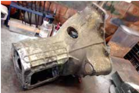
Bare gearbox casing
