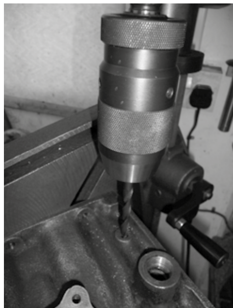
Close up of oil pressure relief valve gallery drilling in side of engine block
