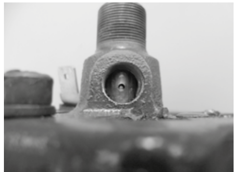
A small hole in the rear bush, visible when the cylindrical brass lubricator is removed, allows lubricant to reach the inner surface of the bush and the rotating spindle.
