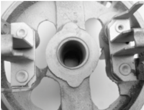
The effects of a worn bush (left top & bottom) compared with those of a brand new bush (right top and bottom). The armature spindle is present in the top (external) views, absent in the bottom (internal) views.
