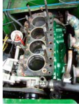
It's not clear but no.1 cylinder is full of water
