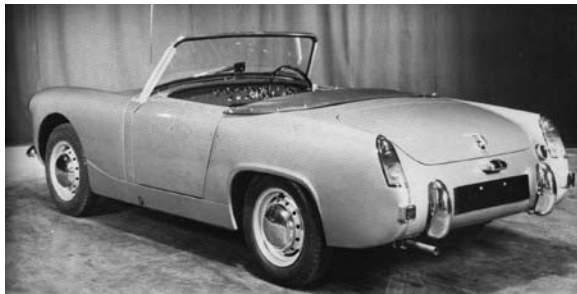
The MkII Sprite prototype photographed at the Cowley studio showing the MG designed rear end. From Geoffrey Healey's book 'More Healeys'
