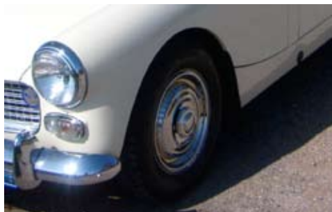
The rare original Ace wheel discs, which were an optional extra on the early Midgets and Sprites
