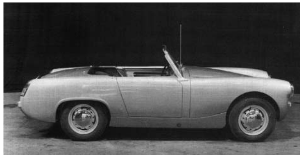
The side on view described in Eric Dymock's book 'The Sprites and Midgets' as the Mark 1½ Sprite. He goes on to say that the tall front wings will be lowered to keep the proportions right before the body dies are made.
