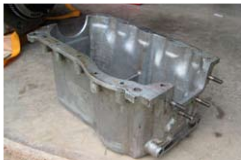
The special aluminium sump
