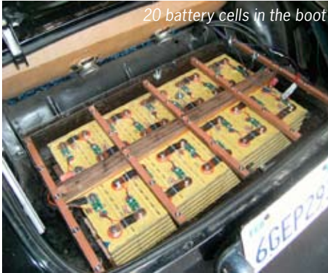
Rear battery box
