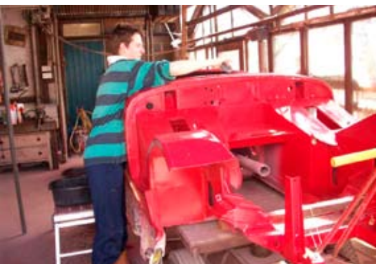
Preparation of the first coats of top coat
