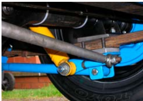
Rear suspension showing the traction bars
