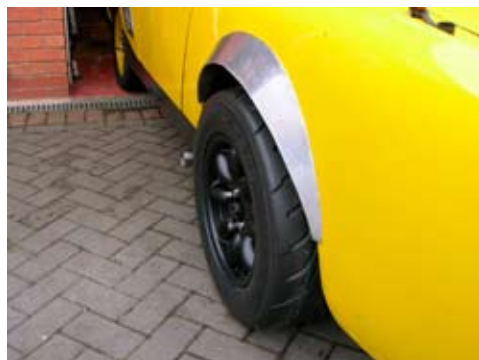
The rear wing extensions, side exhaust and 'sticky' Toyo 888 rear tyres
