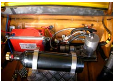
The Nitrous Oxide System gives extra power on tap
