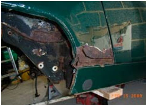
Left spring hanger area – fine example of advanced corrosion!
