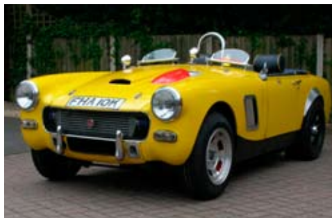
Aero screens fitted, which allow a lunch of flies and bugs
