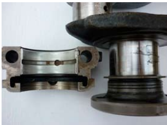
The spiral groove (scroll) at the rear of the crankshaft is here visible lower right. On the left: the rear main cap which is also the lower half of the 'scroll housing'.
