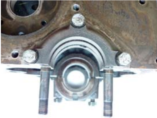
The upper scroll housing (“½ moon” or “eyebrow” piece) is secured by three set screws. It should never be disturbed unless complete reconditioning and line-boring is planned. In this view of the ‘eyebrow’, the rear and middle main caps are absent, the front main cap is positioned loosely.
