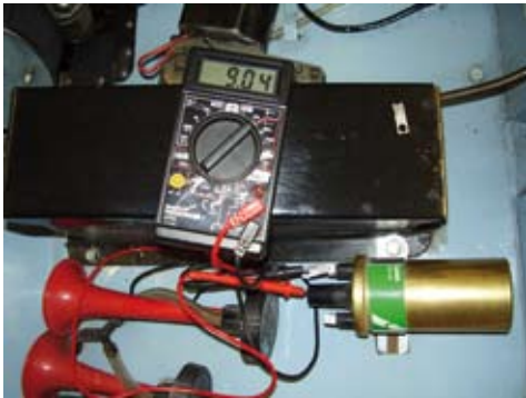
Checking high tension
