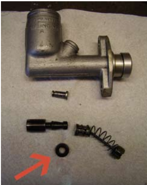
Master cylinder internals showing seal (arrowed) and clevis pin
