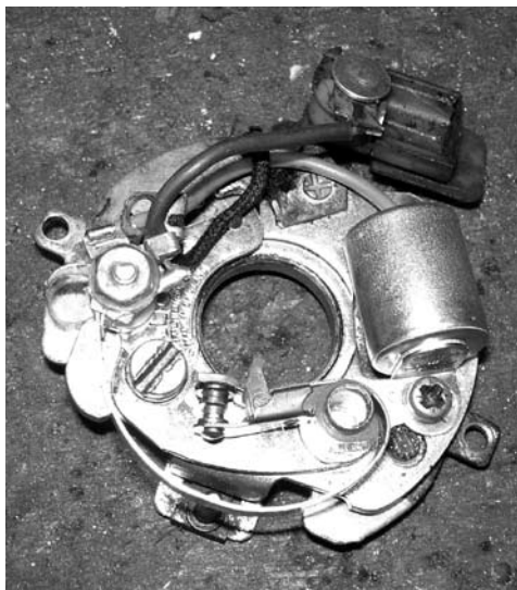
Baseplate set up for roadside replacement
