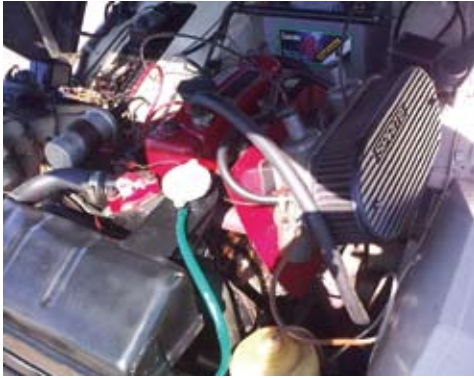
Appearance of cast alloy carb cover far from period, but unbranded air filter (K&N?) works well. Experts say it is more efficient than original pancakes
