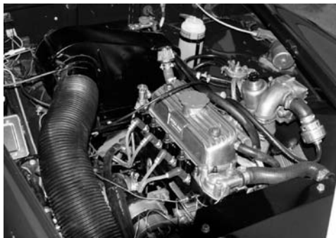
The turbocharged engine of Rob Newton's Midget Mk3
