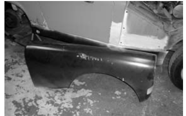
New wing ready for fitting
