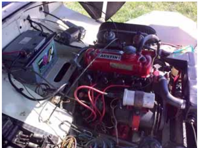
12-volt Dynamo and rev counter drive, tacho gears had to be replaced
