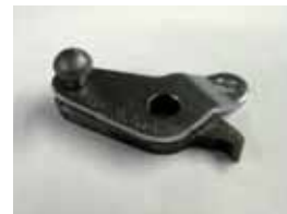
Fig.7 (Right) Locating bracket & rivet on original pawl
