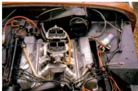
Rover V8 with two 34 DGAS Weber carburetors
