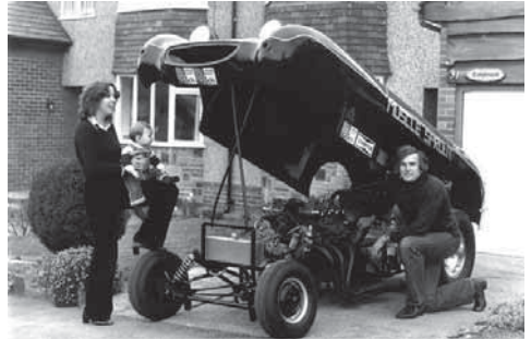
Newly installed Rover V8 engine, with four Weber DCOE two-barrel, side-draft carburetors
