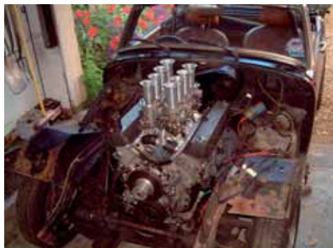
4 x 34 DHLA Dellorto downdraft carburetors (S/H ex Alfa 1.5 Sud/Sprint engines)
