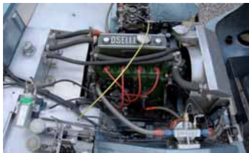
The 998cc Race-prepared engine
