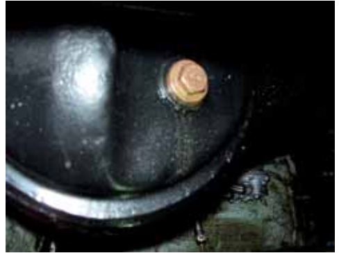
Grubb screw replaced with a brass plug
