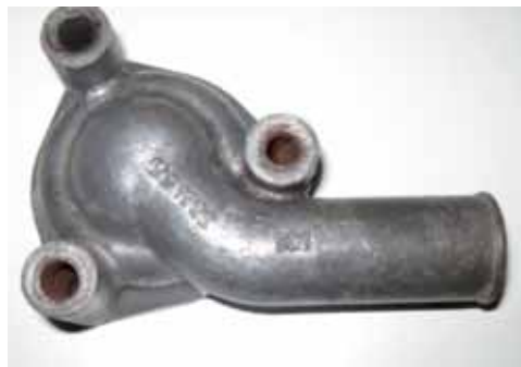
What I believe is the earlier crossflow thermostat housing, this one marked with the part number and DD1 though I have another marked with the part number and DD2
