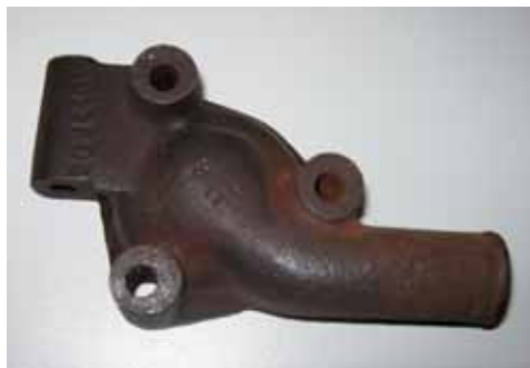
The North American cast iron housing
