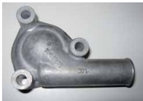
Here is what I believe is the later crossflow housing, this one with identical markings but note the change in style. If you order a crossflow housing new I believe this is the only style still being produced
