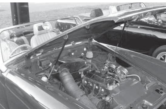
Bonnet supported by struts
