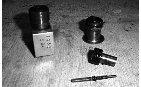
"Broken 90 degree cable drive"
