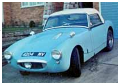
Aluminium bonnet scoop added by Len Pritchard – 1968
