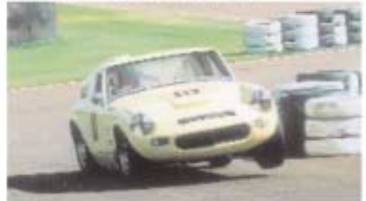
The car lifts a wheel during preliminary testing, which revealed that the suspension required tweaking.
