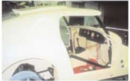
The ledge or the roof for the driver's crash helmet was accurately copied from original 1960's photographs
