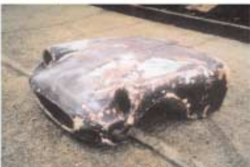
An original Ashley bumper that was repaired prior to a mould being taken from it
