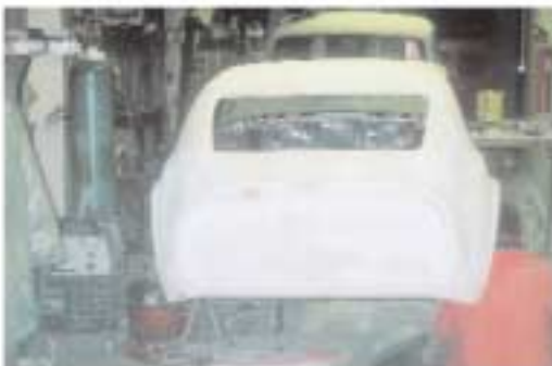
The Lenham GT bodywork is attached to the repaired floor pan
