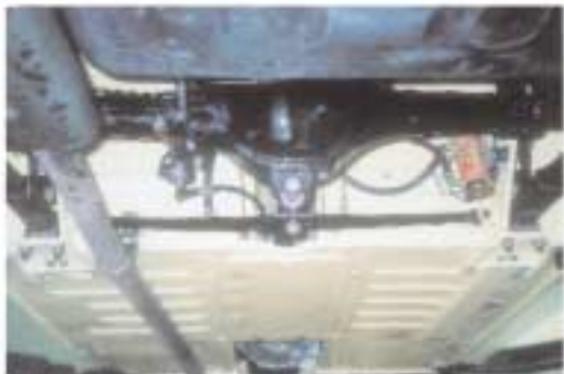
An "A" frame like the one Oliver had made for BRCC's original car (note: the back axle
