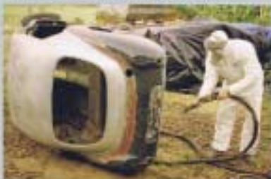
▲ Paul Woolmer had completed a small amount of restorative work, which had centred around getting the bodywork sandblasted in readiness for the bodywork repairs.
