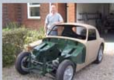
▲ Ironically, Dave completed the spray of the car in his garage at home. The body was silt-primed and then finished in British Racing Green using cellulose paint.
