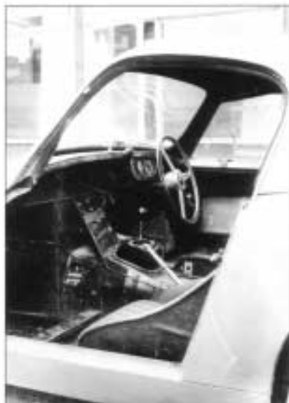
Left: The stripped out interior of S 221 during 1961. Healey glass fibre seats, 3-spoke wooden steering wheel, small dash and Speedwell instrumentation, were standard fitment on all W&P alloy coupes. Below: 46 BXX racing at Brands Hatch during 1961.
