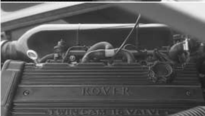
MCF-ported E-Series is a neat fit in the Midge — even the standard bonnet remains.
