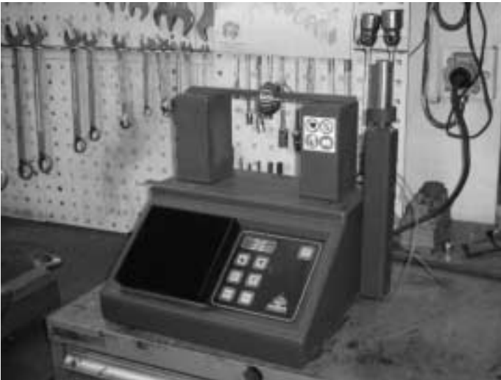
Bearing heater at 36°
