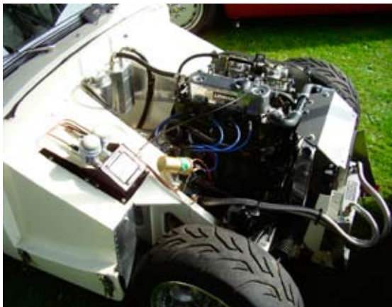
The Lenham Motor Co's Lenham Le Mans Sprite Engine and under-bonnet concealed wiring
