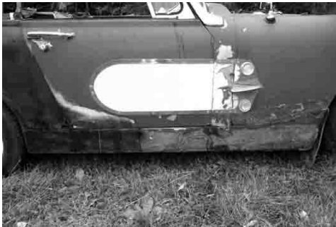
Clearly visible signs of the remains of the special equipment side pod
