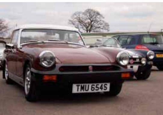
Andy Harrison's low 1500 Midget. It has a Frontline front end (springs and top link kit) and lowering blocks on the back
