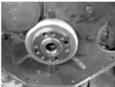
Oil seal seated in housing
