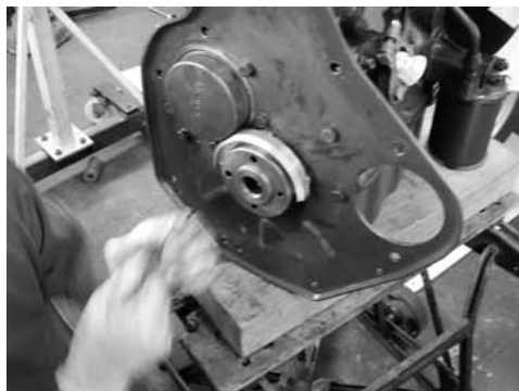
Top half of seal housing in situ
