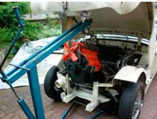
It's so much easier with a Frogeye! Compared with the later cars, the required lift is much lower and the required tilt is much less dramatic
