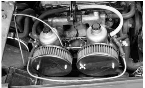
New air filters in place
