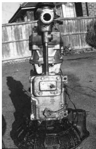
The overdrive-enhanced Triumph gearbox
