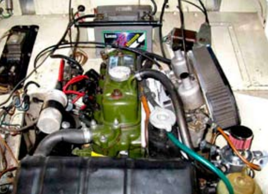
Shiny aluminium oil catch tank is well made, but like the aftermarket air filter is another non-original fitting
