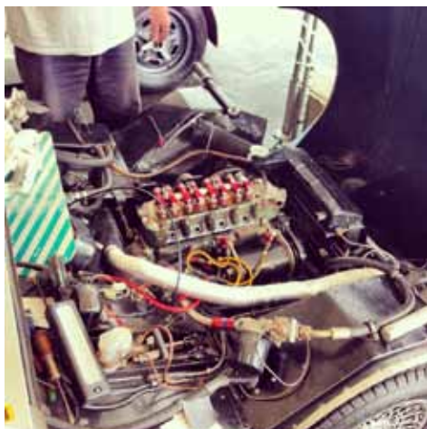
Engine back together with new head gasket after blowing up on the Mulsanne straight
